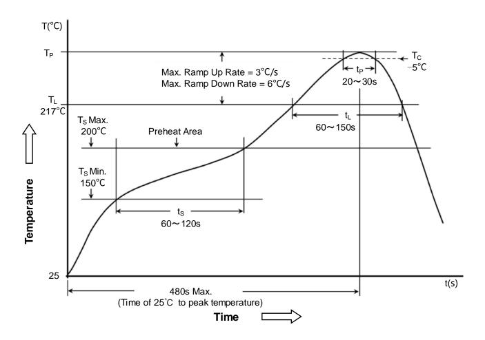
8.2 Classification of Peak Package Body Temperature (T<sub>P</sub>) 封装体峰值温度(T<sub>P</sub>)分类
